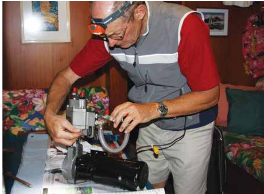
Watermaker servicing above; view of the Frigoboat refrigeration system, below
